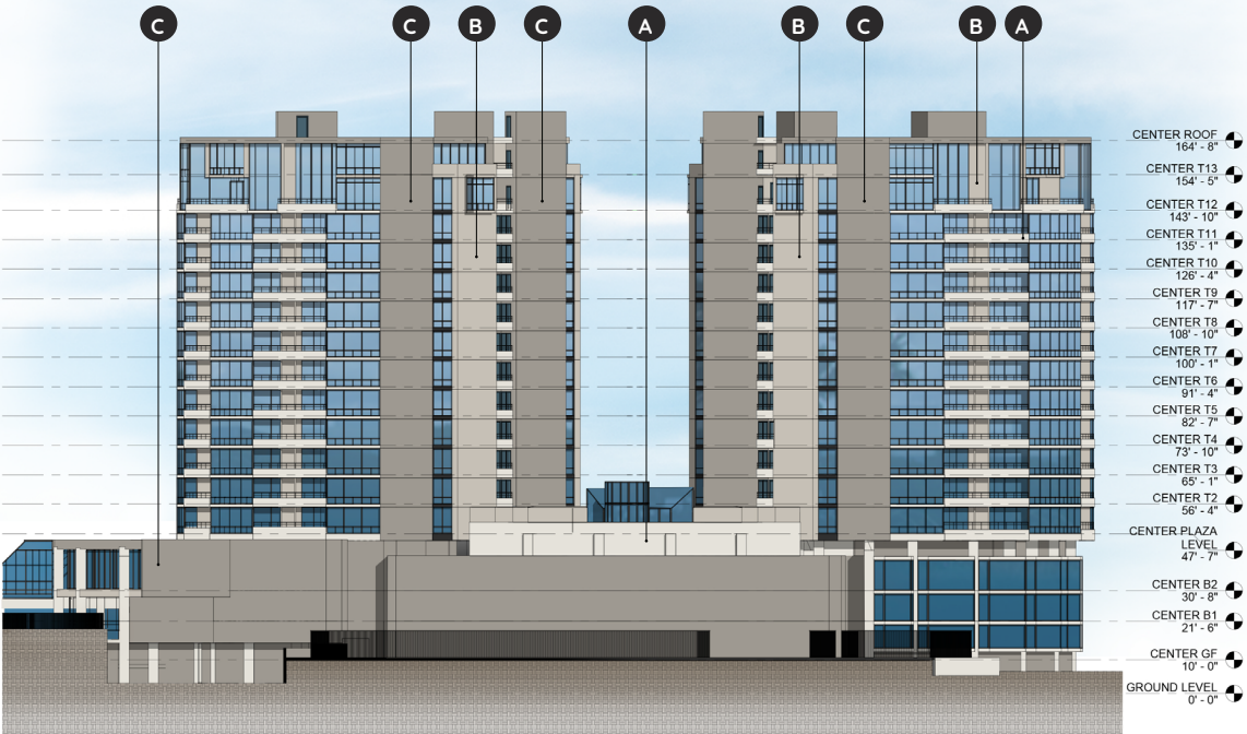
A2 - CENTER TOWER - EAST ELEVATION
