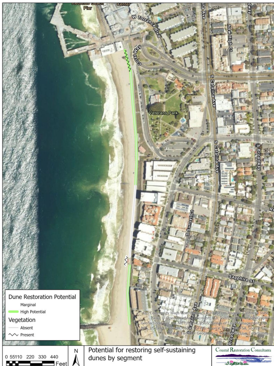
Figure 2-27. Potential for restoring self-sustaining dunes at Redondo Beach
