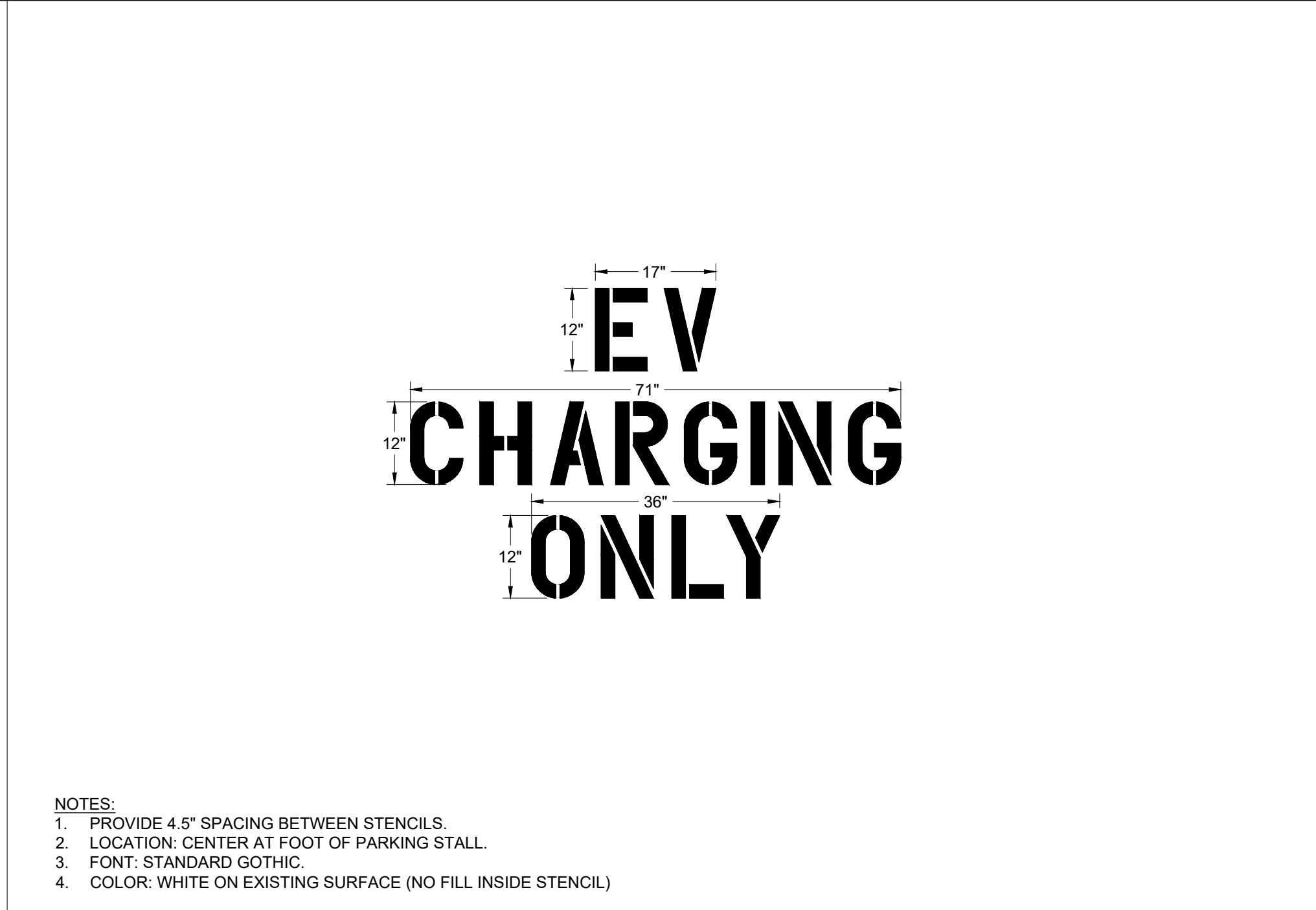
4 ELECTRIC VEHICLE ONLY SURFACE STENCIL DETAIL NOT TO SCALE
