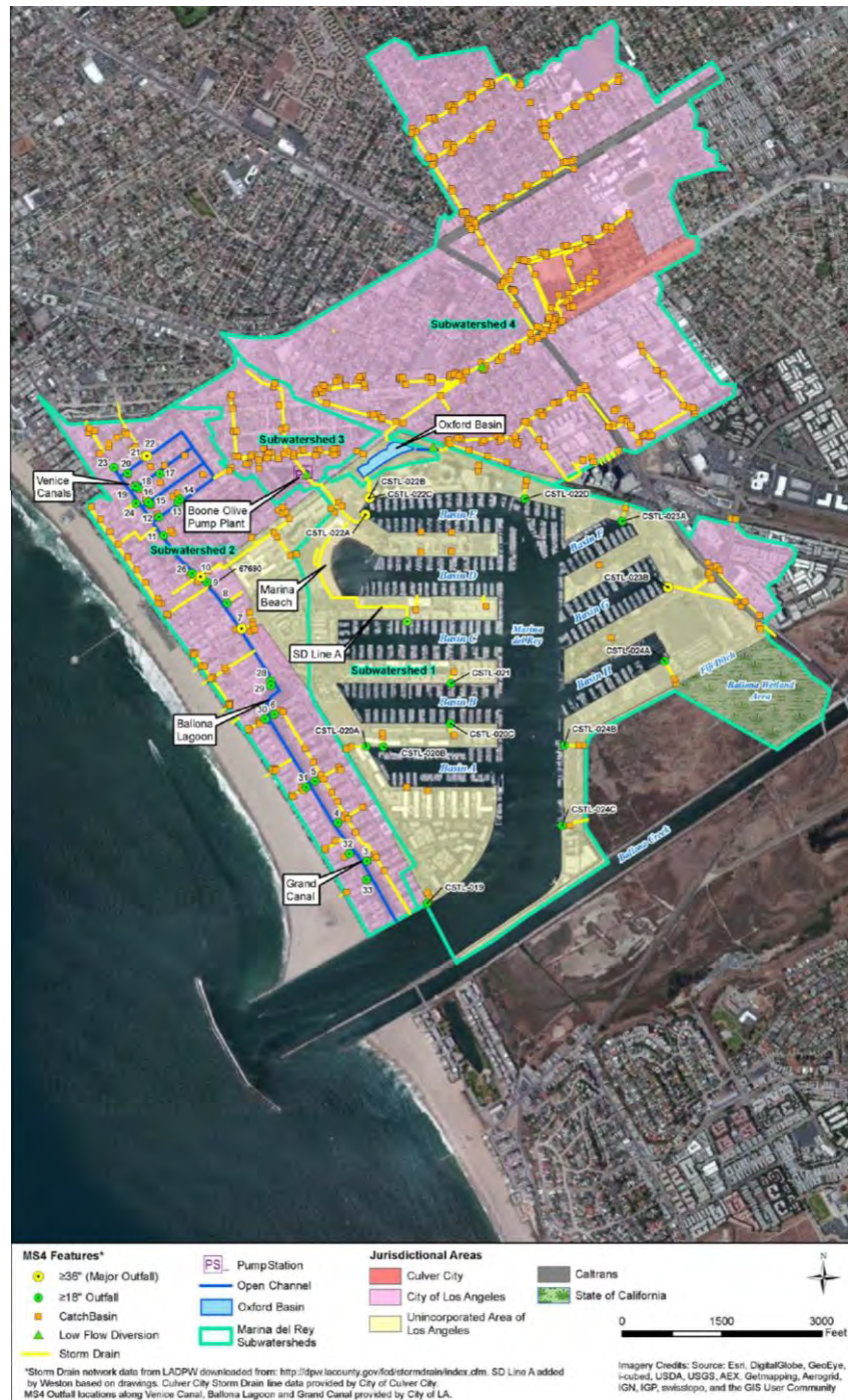
Figure 4. Storm drain and outfall locations (adapted from Figure 1-1 in the Marina del Rey Coordinated Integrated Monitoring Program document, February 29, 2016).
