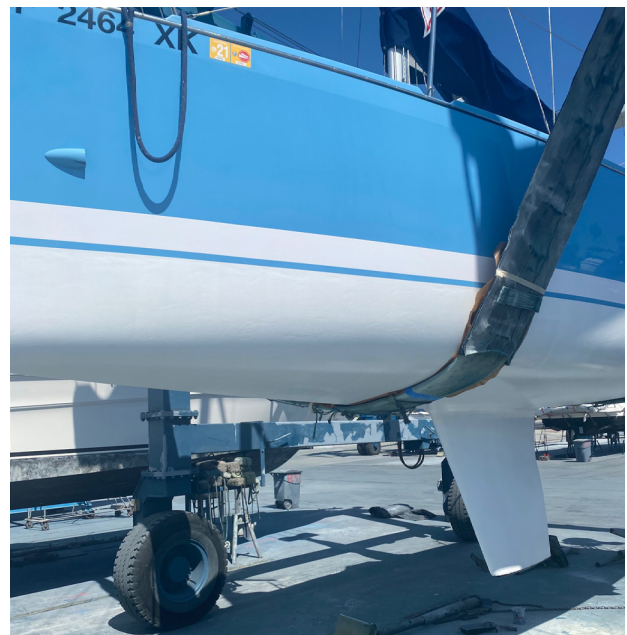
Non-biocide paints being applied to two County-owned vessels.
