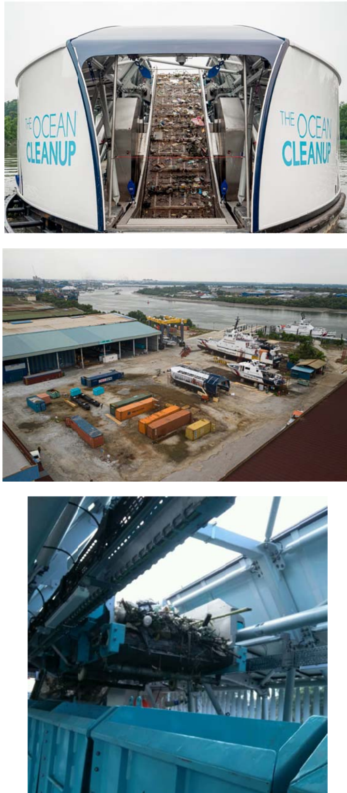
Figure 2. Pictures of Interceptor™ barge in Malaysia with barrier and dumpster barge.
