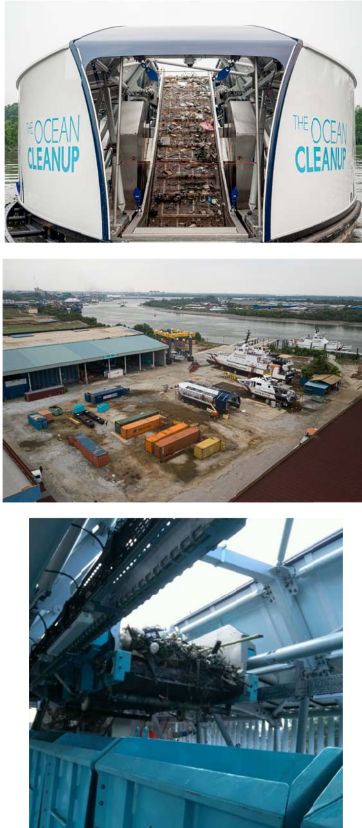
Figure 2. Pictures of Interceptor™ barge in Malaysia with barrier and dumpster barge.
