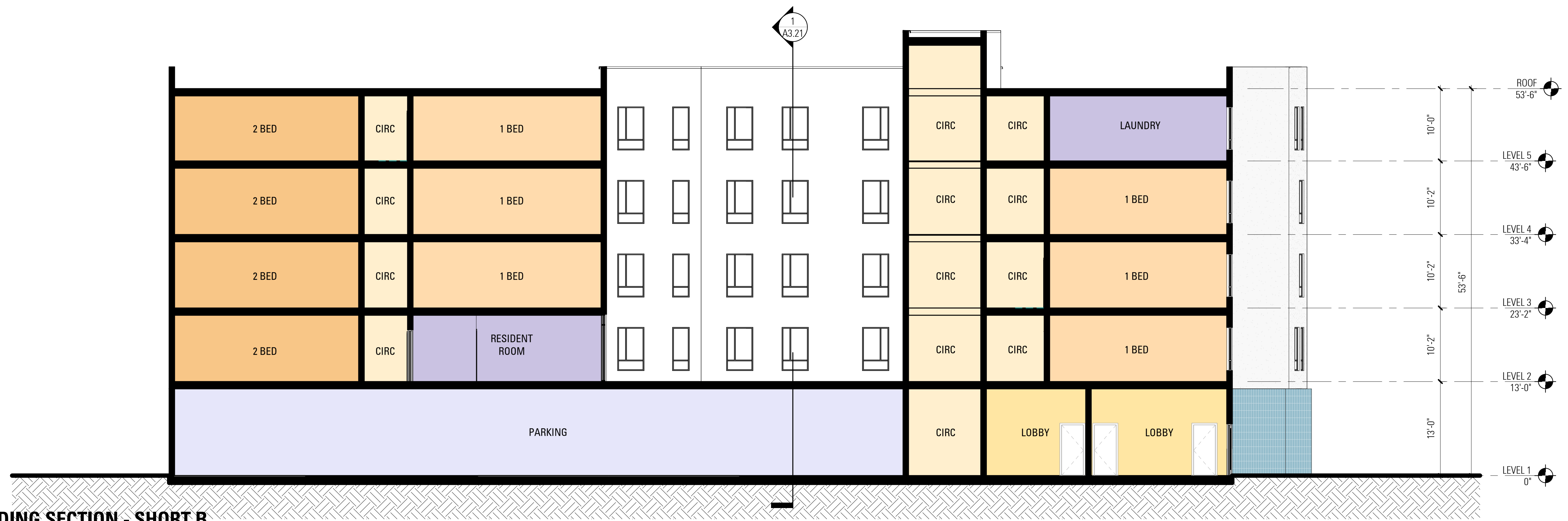
BUILDING SECTION - SHORT B 3 A3.21 1/8" = 1'-0"
