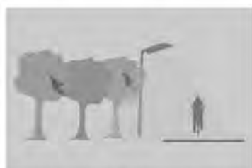
Figure 5.4. Avoidance of light trespass by installing shielded luminaires. Left - conventional luminaire with light spillage into the adjacent forest habitat, right - shielded luminaire that focuses the light cone only on the area where it is needed (© H. LIMPENS).
