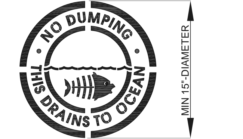
STORM DRAIN STENCIL DETAIL NOT TO SCALE
