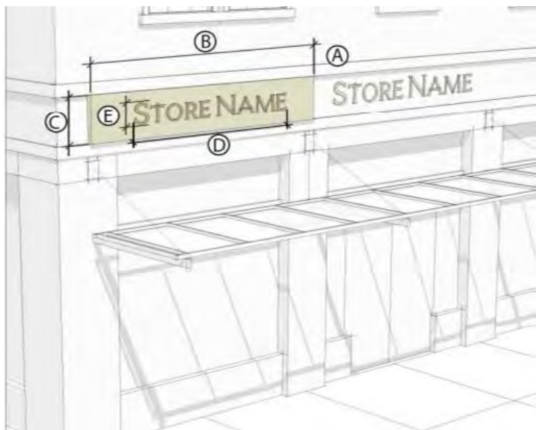
FIGURE 22.366.090-H: PROJECTING SIGN DESIGN
