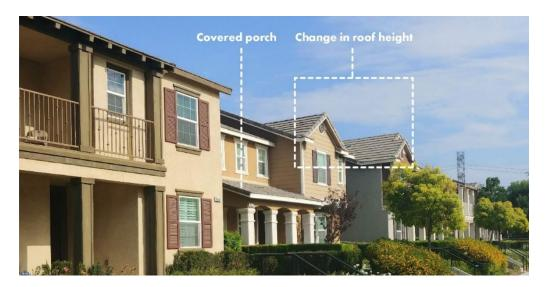
Figure 2-29 Entryway projection with balconies. Marina Del Rey, CA. Source: Gruen Associates
