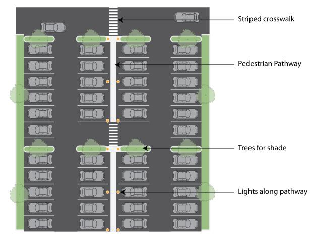
Figure 2-116 Surface parking lot with pedestrian friendly amenities. Source: Gruen Associates
