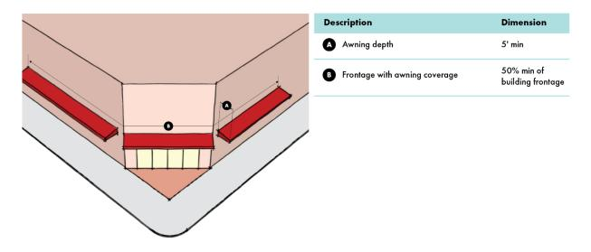
*Figure 2-63 Five-foot-deep awning covering 50% of the building frontage. Source: Gruen Associates*
