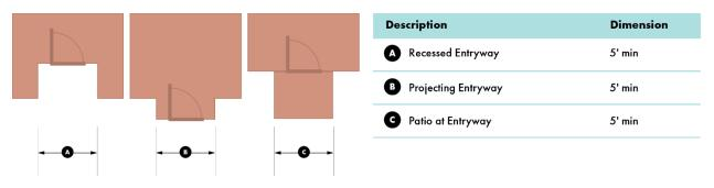
Figure 2-12 Entryway width for Single-Unit or Multi-Unit (Private entry). Source: Gruen Associates
