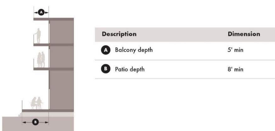
FIGURE 22.140.520 – L: Cantilevered, semi-recessed, and recessed balconies.
