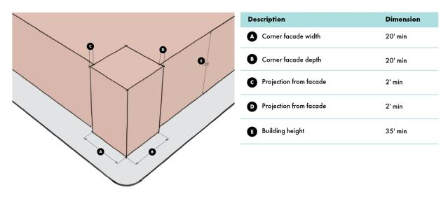
Figure 2-52 Corner façades popping out at the corner. Pasadena, CA. Source: Gruen Associates
