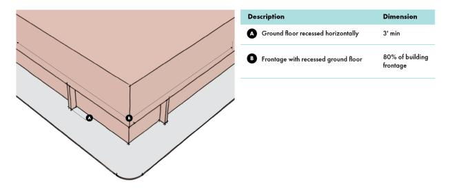
Figure 2-62 Recessed ground floor. San Pedro, CA. Source: Gruen Associates
