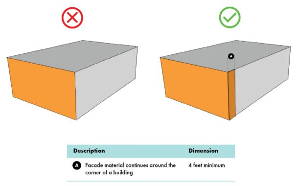
Figure 2-71 Façade material and color changes. Examples from Pasadena, West Hollywood, and Los Angeles. Source: Gruen Associates.
