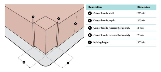
Figure 2-50 Corner façades recessed from taller tower. Santa Monica, CA. Source: Gruen Associates
