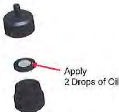
Figure 4-4: Apply 2 Drops of Oil to Impactor Plate
