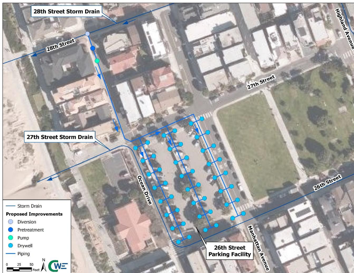
Figure 2-2 Phase 1: 26 th Street Parking Facility Drywell Concept
