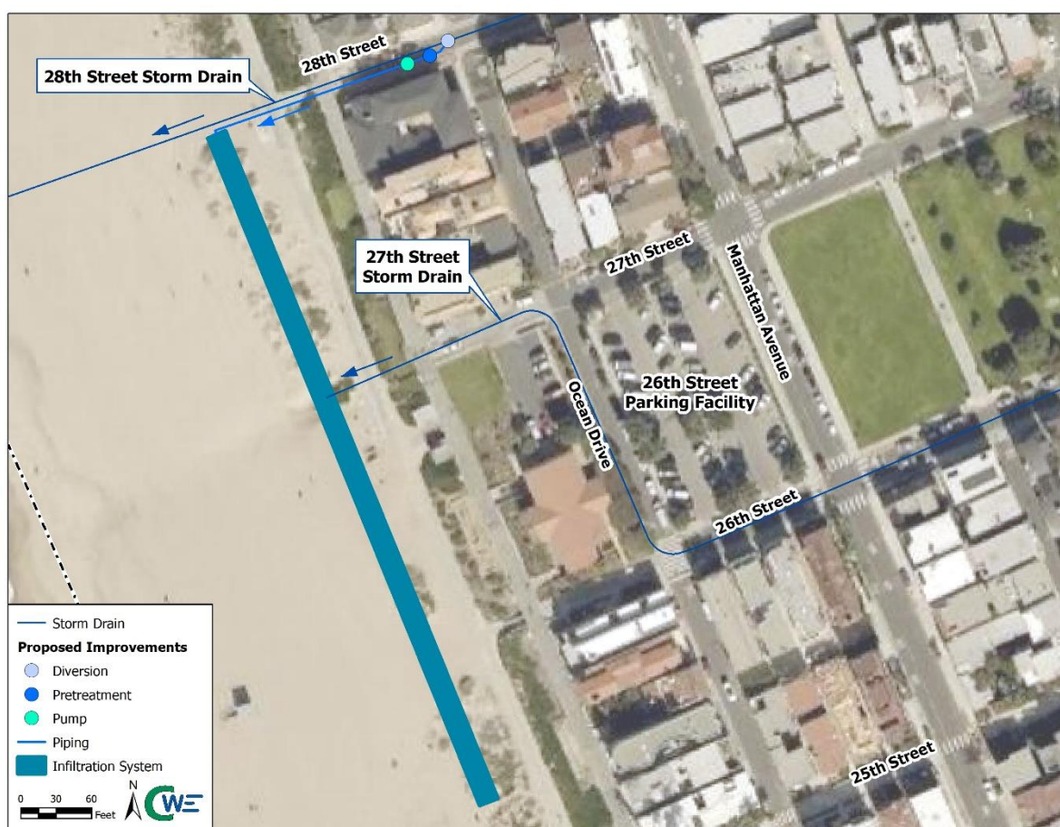
Figure 2-3 Phase 2: Beach Infiltration Concept
