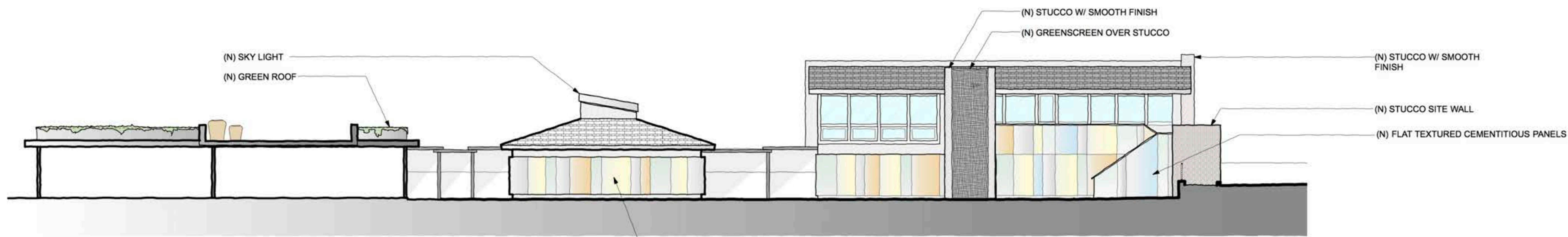
proposed leasing building improvements - north elevation scale: 1/8" = 1'-0"
