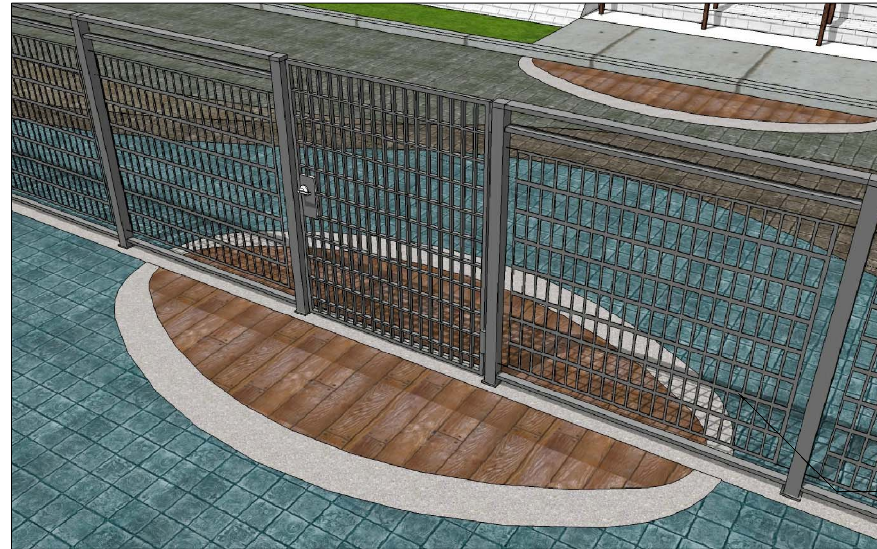
PROMENADE FENCE BY CRANEVEYOR CORP. NO OF GATES = 7 TOTAL LENGTH OF 6" HIGH FENCE = 1230'
