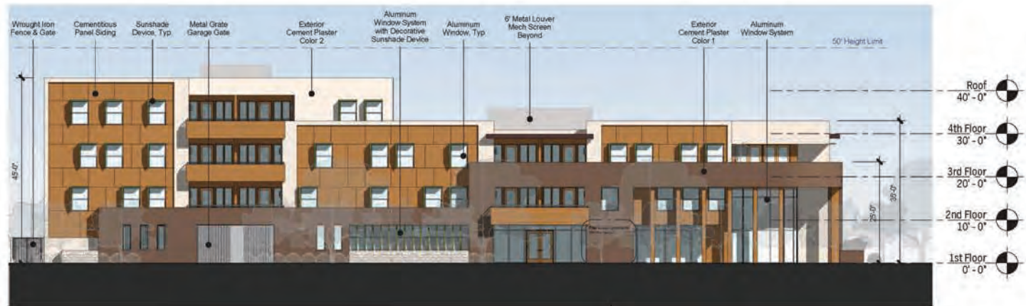
② West Elevation - Peck Road Elevation 1" = 10'-0"
