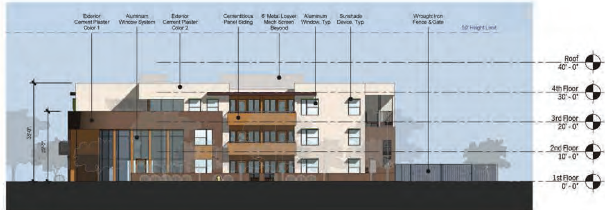
① South Elevation - Ranchito Street Elevation 1" = 10'-0"
