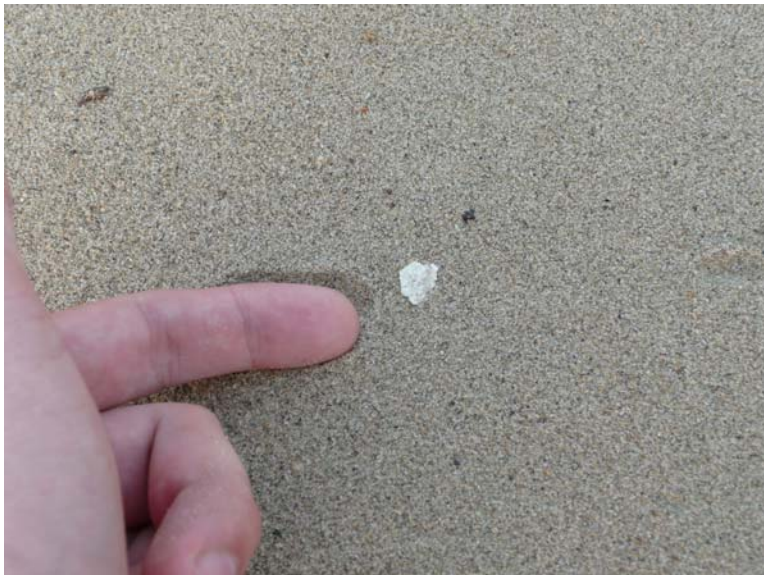
Figure 6 – EPS fragment not collected by the sanitizer beach cleaning machine at Venice Beach
