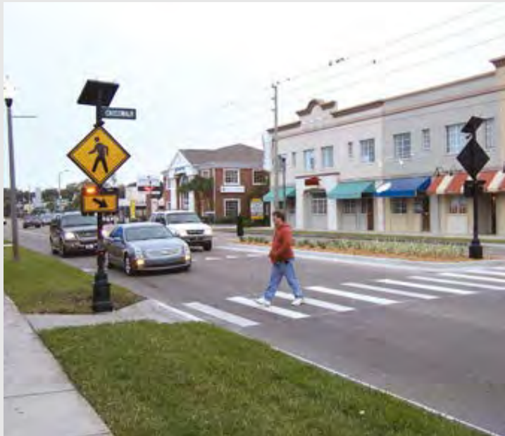
Rapid Flashing Beacons
