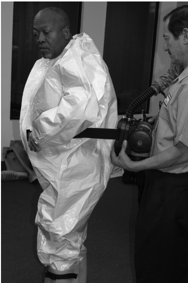
Step 4 – PAPR belt Don the respirator belt or vest. Don the battery and turn it on.
