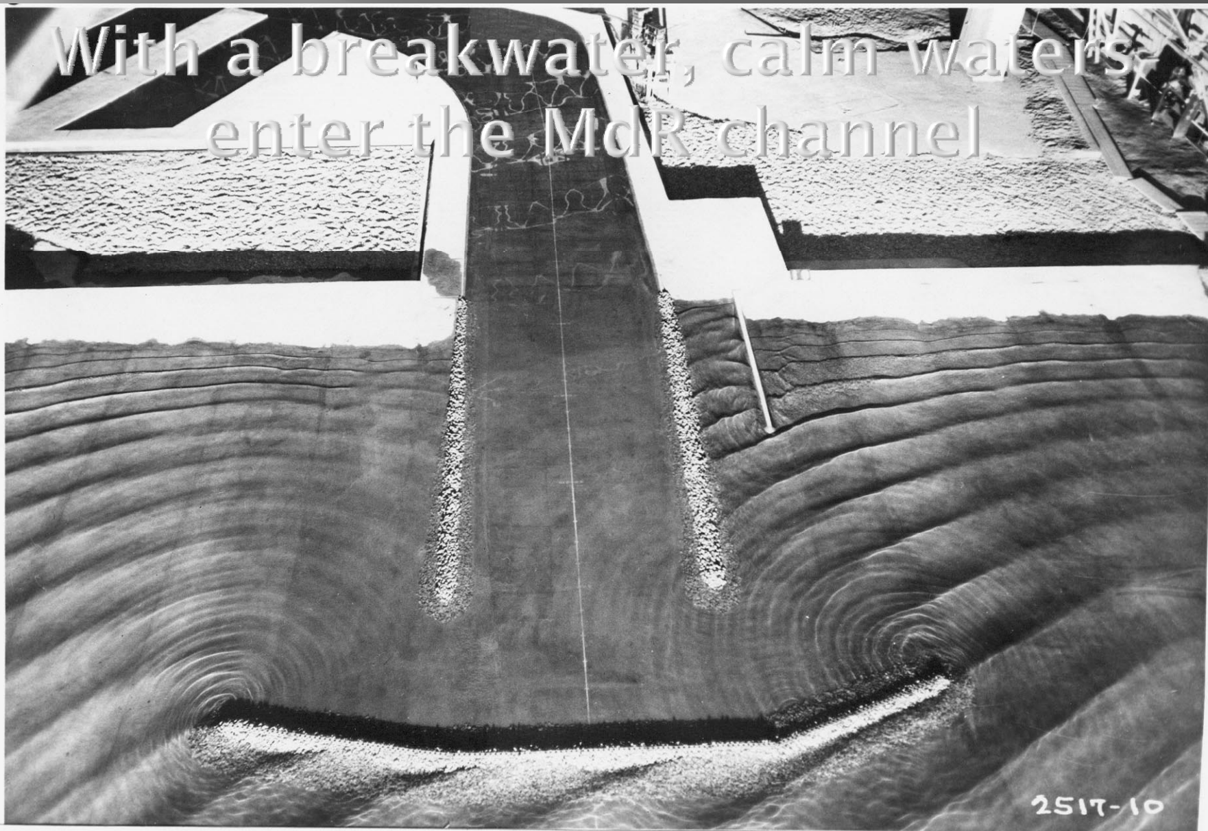
U.S. Army Engineers test model of MARINA DEL REY showing wave action in harbor with breakwater 8 SECOND INTERVALS 8 FOOT WAVES 30° SOUTH CENTER LINE = 0°
