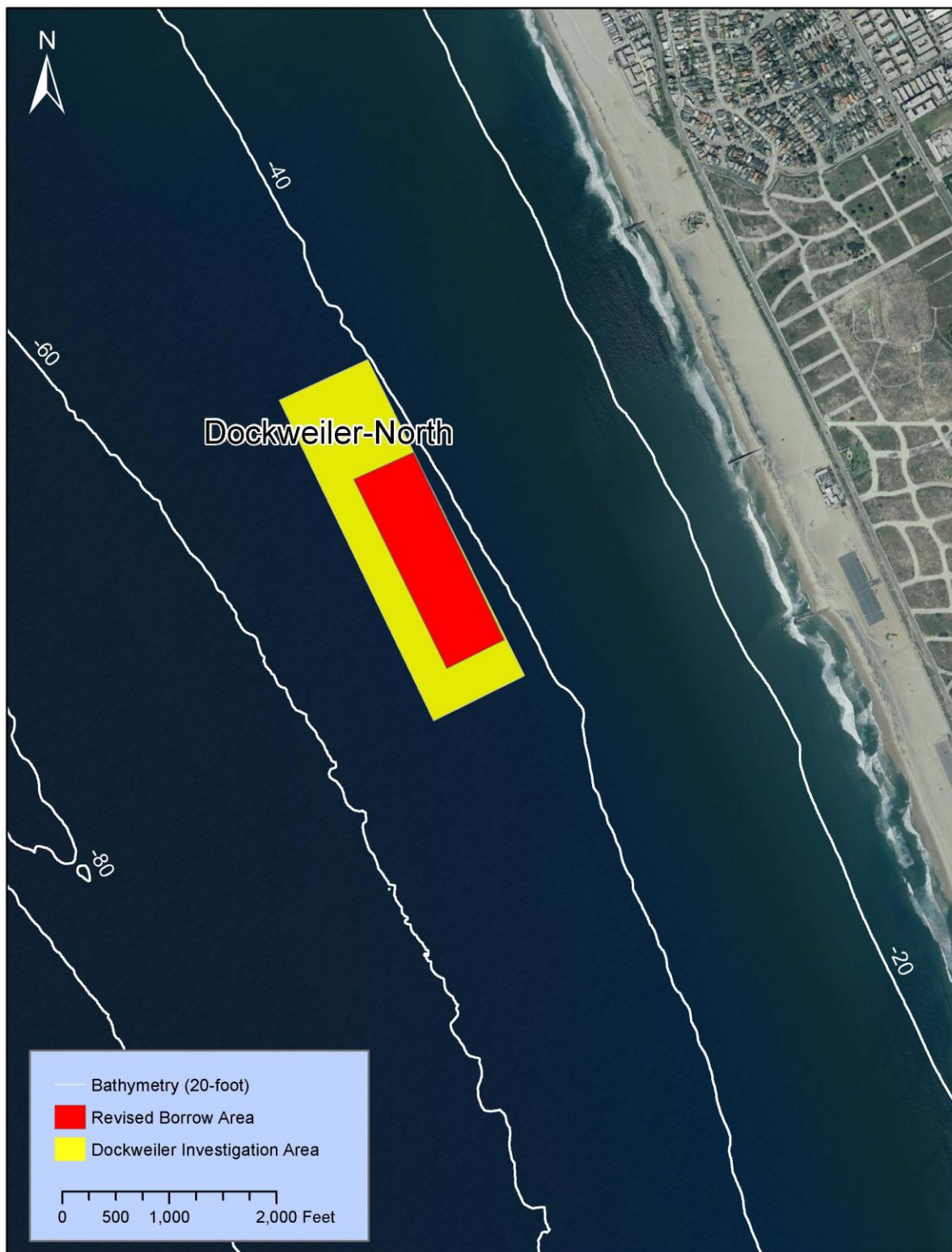
Figure 14. Dockweiler Offshore Sand Investigation Area And Target Dredge Area
