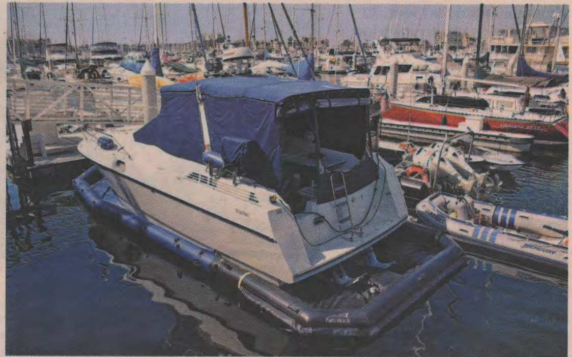
This Fab Dock is being tested out at a slip at Anchorage 47 in Marina del Rey Harbor as part of research into solutions to reducing copper levels in the water.
