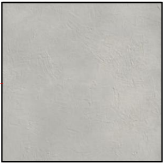
(CT-3): CEMENT/ RESIN SLAB FLOORING EXTERIOR RATED, SLIP-RESISTANT AT RECESSED ENTRY ALCOVE FLOORING
