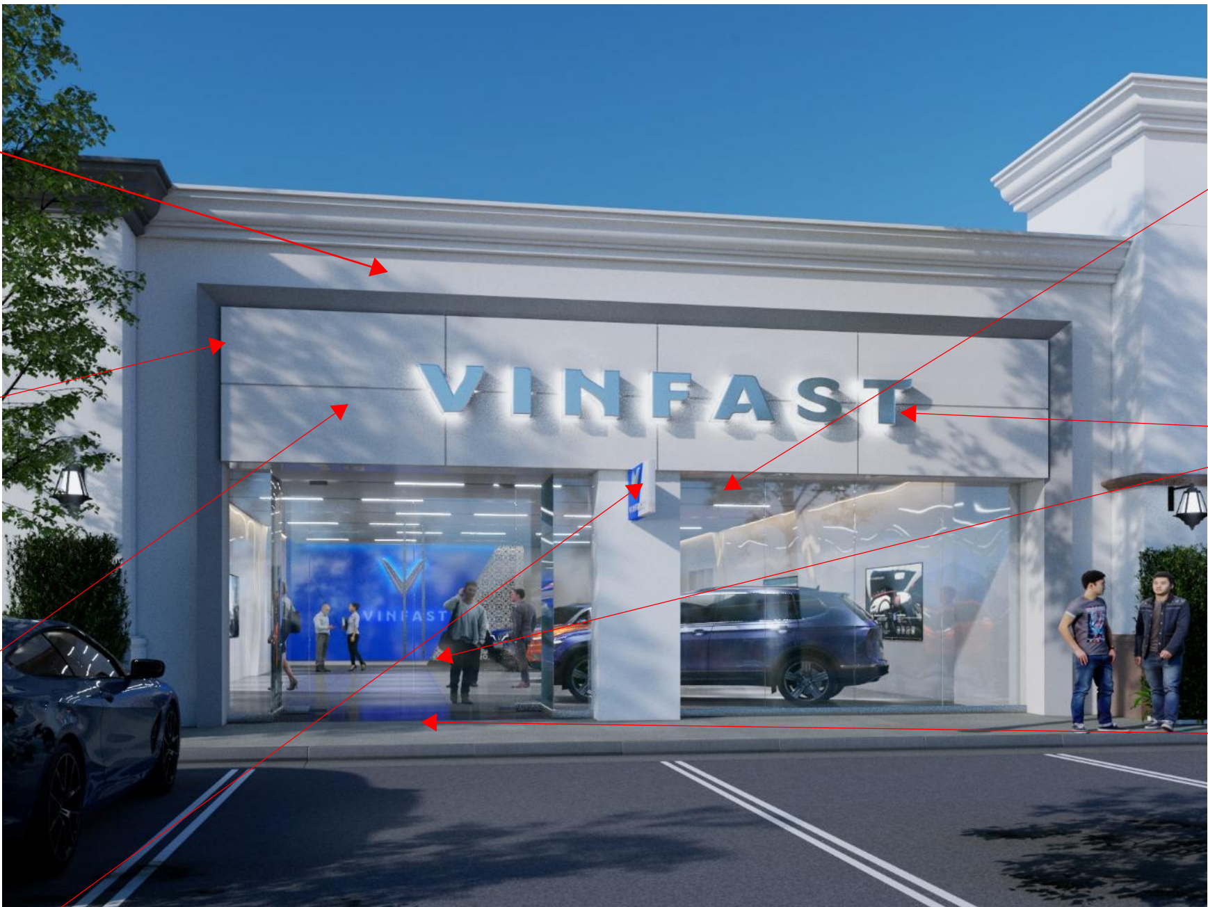
(PT-2): SHERWIN WILLIAMS CUSTOM TO MATCH PANTONE COOL GREY 9C AT (E) ANGLED STONE PORTAL FRAME
