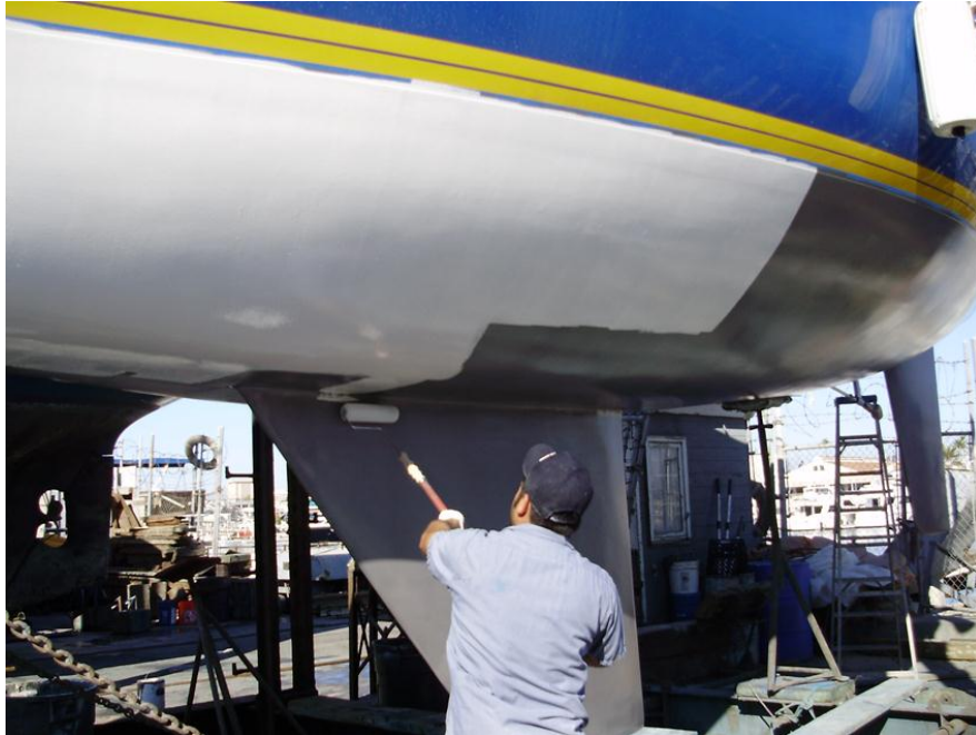
Figure 5-30. Painter Applying Sealer
