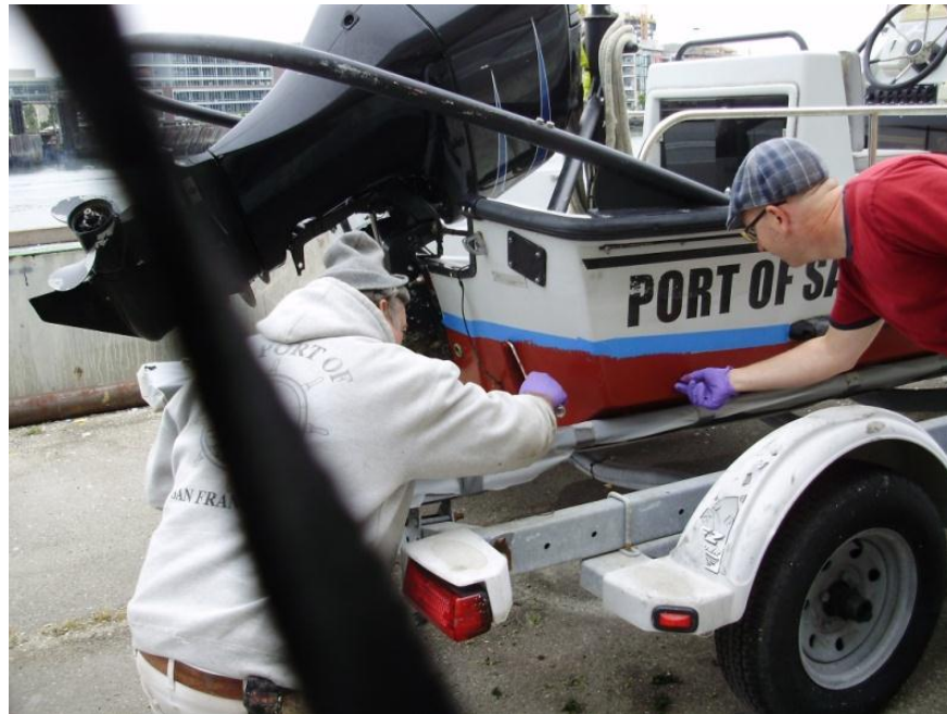
Figure 5.9. Port of San Francisco During Paint/Hardener Touchup Operation
