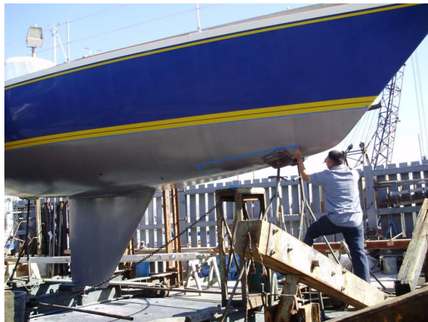
Figure 5-31. Painter Applying Intersleek 900 Topcoat
