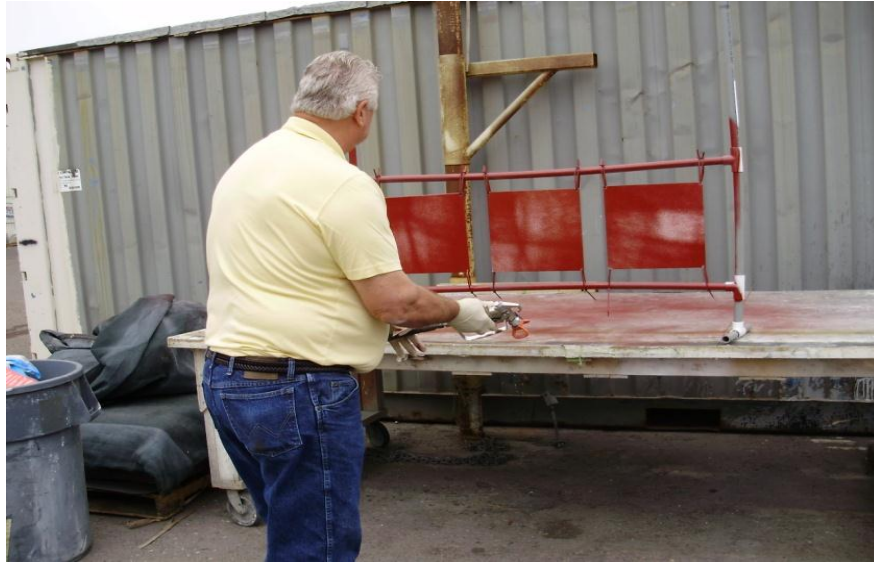
Figure 3-3. Supplier Spray Painting Panels
