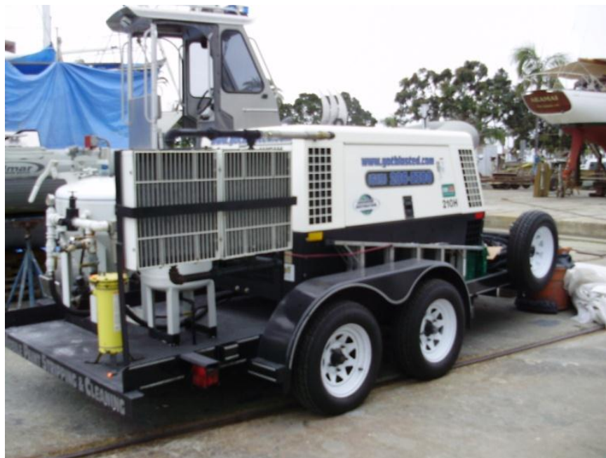
Figure 5-27. Sodium Bicarbonate Stripping System at Boatyard
