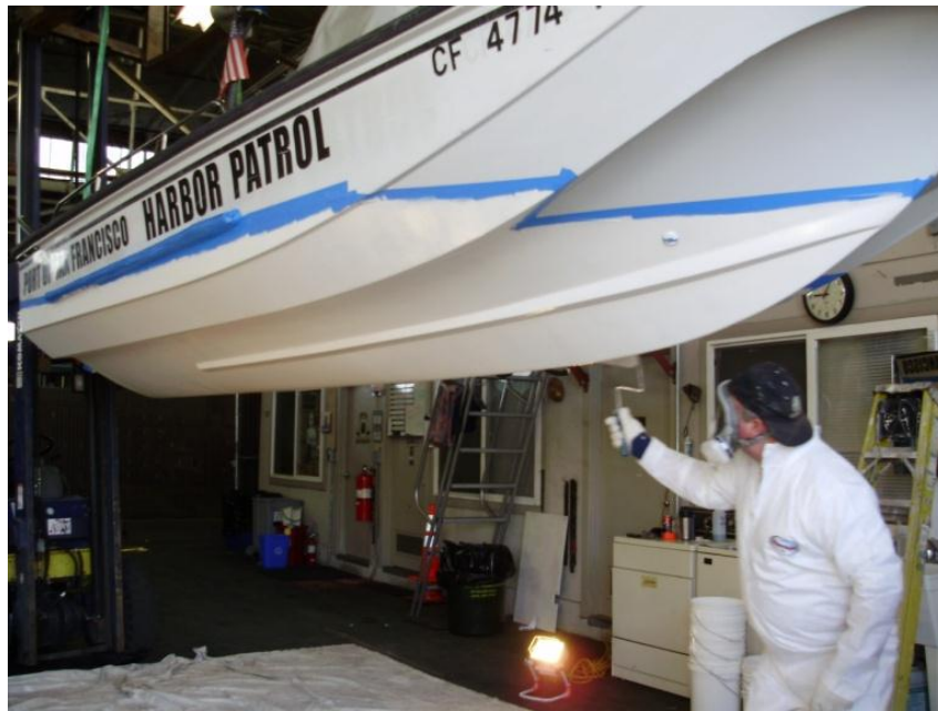
Figure 5-4. Painter Applying Tiecoat.
