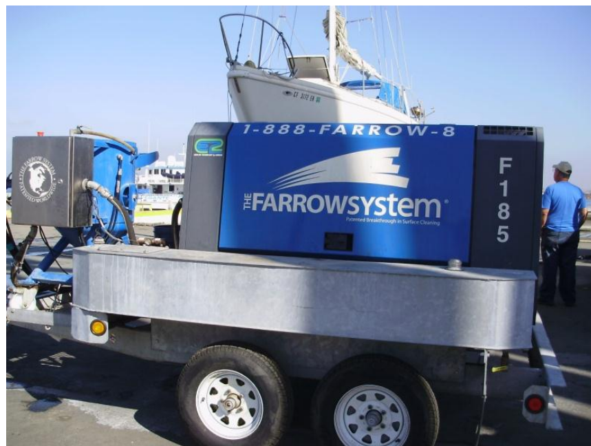
Figure 4-2. Volcanic Rock Blasting System
