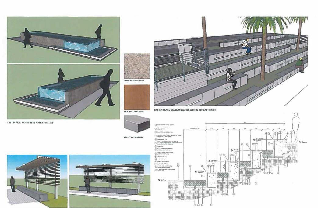
CAST IN PLACE CONCRETE BENCH WITH ALUMINUM AND WOOD COMPOSITE TRELLIS, VINES TO BE TRAINED TO GROW UP POSTS
