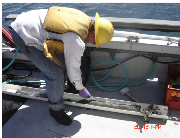
Figure 6. Geologist cutting polyethylene liner prior to logging the core's lithology.
