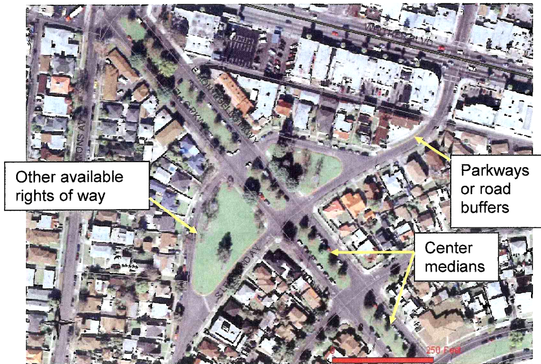
Figure E: Storage in road right of way
