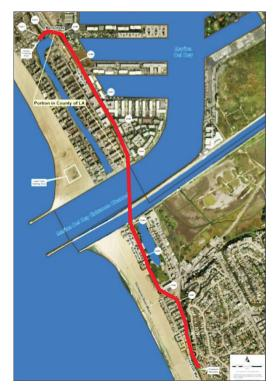
The sewer will originate at the Venice Pumping Plant located on Hurricane Street and cross Grand Canal, travel east to Marquesas Way, then south along Via Marina crossing the Marina del Rey and Ballona Creek Channels to meet an existing Coastal Interceptor Sewer on Vista del Mar near Waterview Street.
