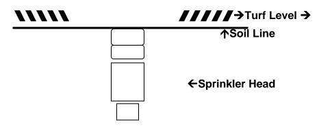
2. Standard sprinkler head installation with consideration for the thatch and mat accumulation. . . .
