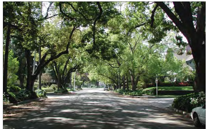
Street trees reduce the visual width of this 40-foot wide street and, along with the mottled pattern of dark and light that is cast on the roadway, encourage motorists to slow down.
