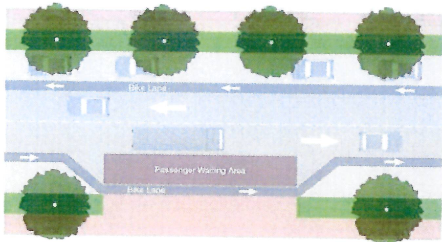
Figure 4.3 Floating Bus Stop And Bike Channel Design
