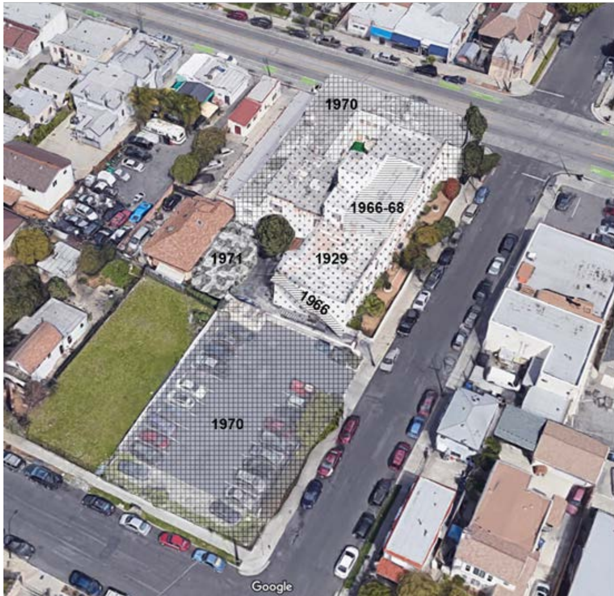
Figure 5. Schematic Diagram of Japanese Hospital, indicating dates of construction or alteration to the various components of the building. (Little Tokyo Historical Society, 2015)
