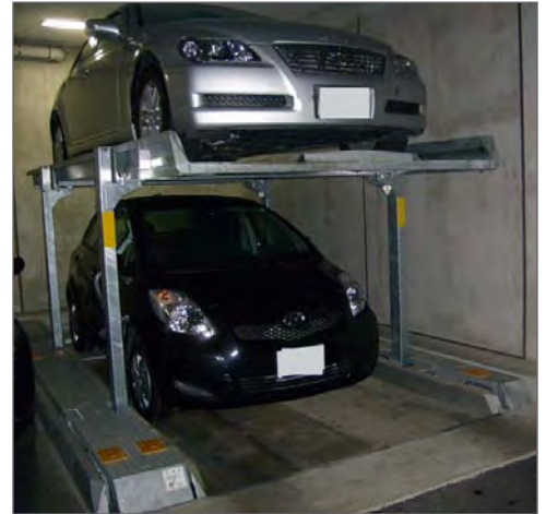
Garage lifts (stacked) parking may help to increase the capacity of a parking structure.
