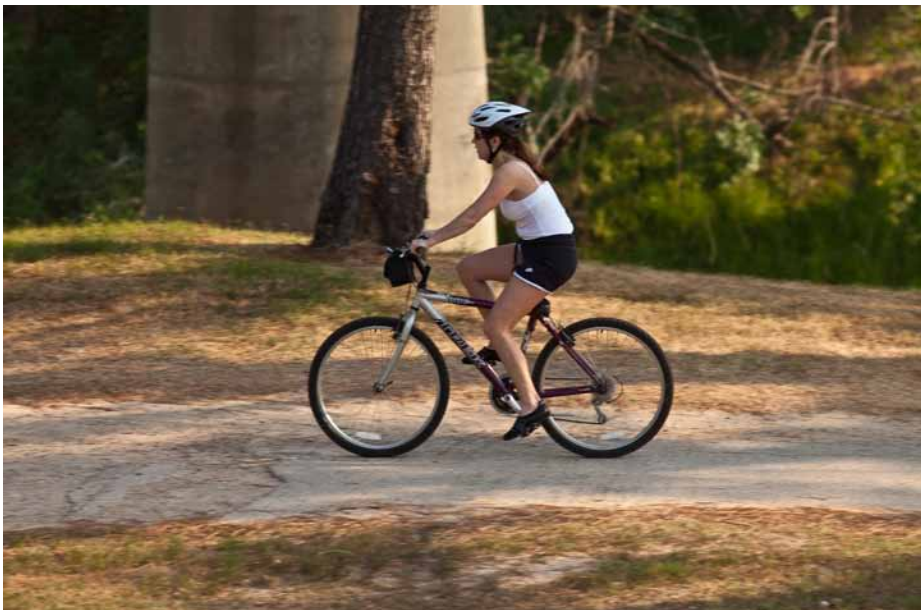
Bicycle path on stabilized decomposed granite
