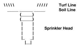
2. Standard sprinkler head installation with consideration for the thatch and mat accumulation. . . .
