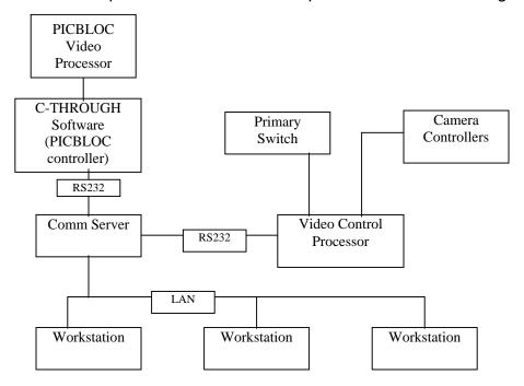
All commands to the CVCS originate at the operator workstations. The commands are sent to the communication server through the LAN. Based on the specific command, a process in the communication server formulates one or more specific commands for the video components. The commands are sent via RS232 connection to either the video control processor or the computer on which the C-THROUGH software operates.
