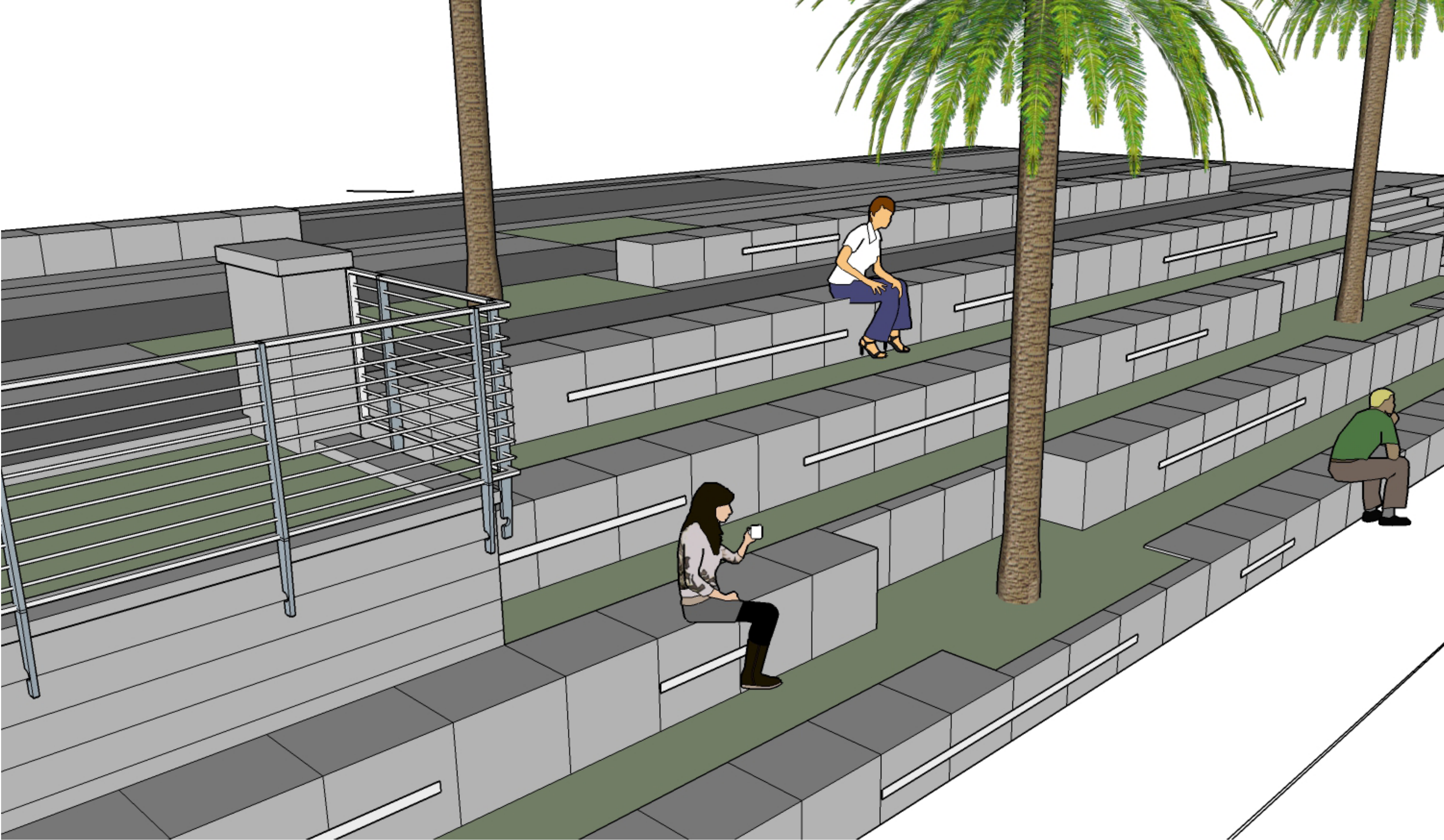
CAST IN PLACE STADIUM SEATING WITH #3 TOPCAST FINISH
