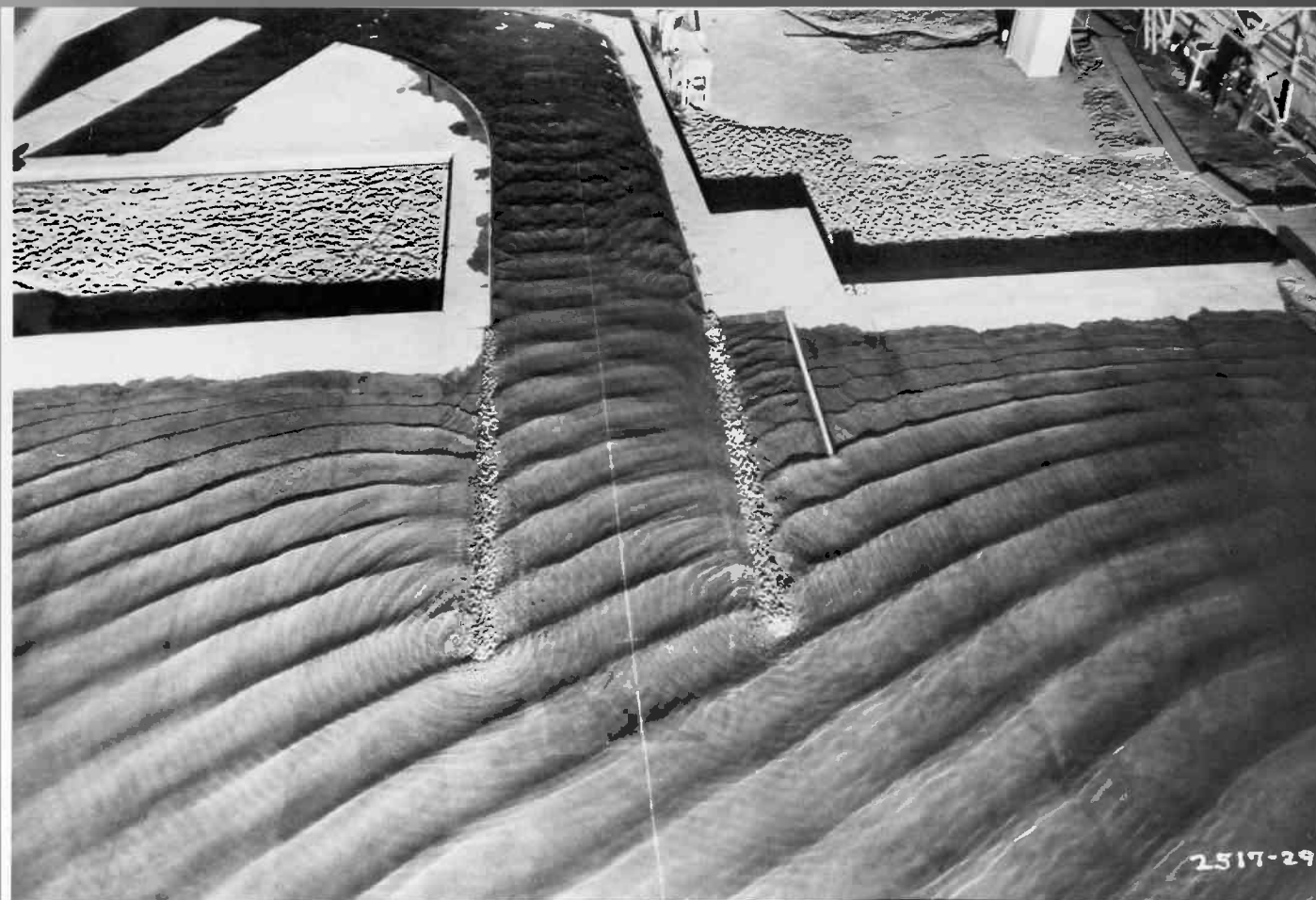
U.S. Army Engineers test model of MARINA DEL REY showing wave action into harbor without breakwater 8 SECOND INTERVALS 8 FOOT WAVES CENTER LINE = 0°
