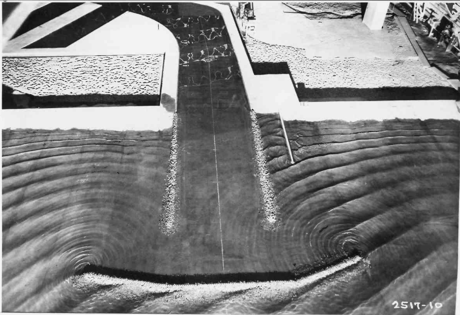
U.S. Army Engineers test model of MARINA DEL REY showing wave action in harbor with breakwater 8 SECOND INTERVALS 8 FOOT WAVES 30° SOUTH CENTER LINE = 0°
